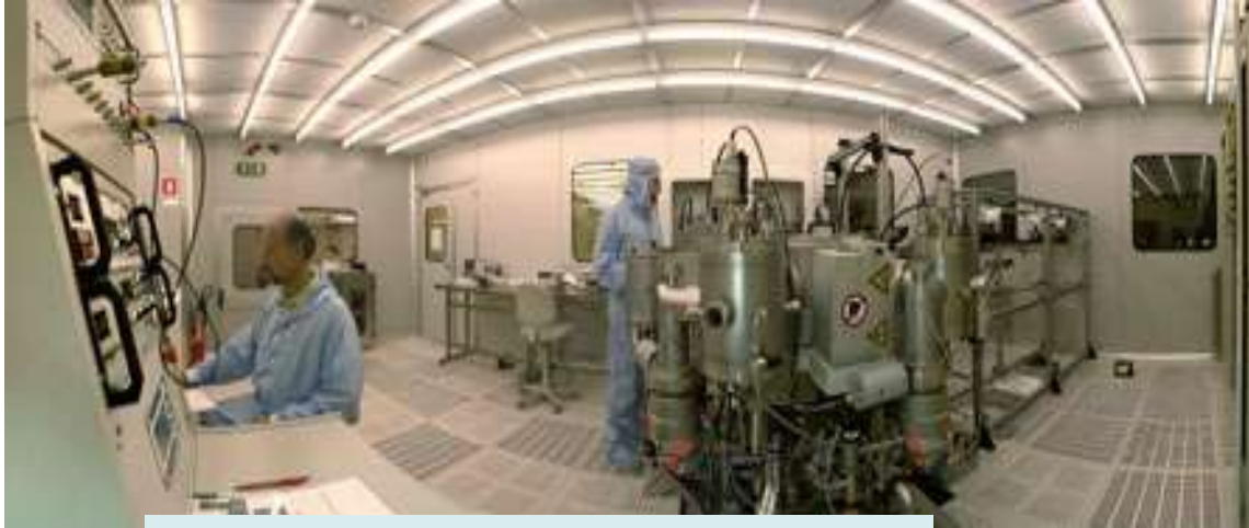
Clean room for photolithographic process
