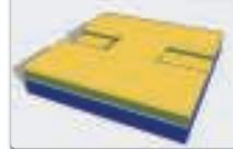
Electrode metallization by sputtering or evaporation
