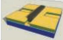
Gate support is created by ion beam induced metal deposition
