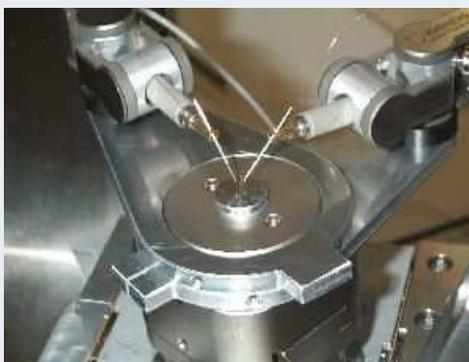
Two Micromanipulators mounted on the specimen stage.
