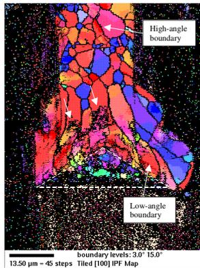
OIM image of the wire bond cross-section. A deformation concentration can be noticed (dashed line triangle). Thick lines are used for high angle grain boundaries ( $>15^\circ$ ) and thin lines for low angle boundaries ( $<15^\circ$ ). The arrows point on the contamination visible on the FIB image.
