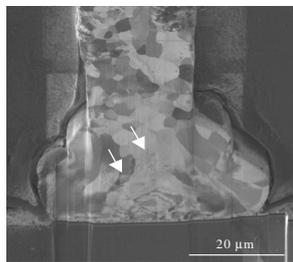
FIB image of the cross-section of a Cu wire bond prepared by polishing and FIB milling.
