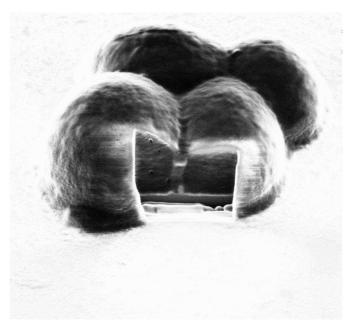
FIB Images of two adhering yeast cells after being cut by the ion beam. It is possible to see inner structures of yeast, details of the membrane-wall complex, details of the adhesion of cell to substrate. The precision of the orthogonal planes sectioning can be appreciated, together with the resistance of the cellular structures to the vacuum chamber operation.
